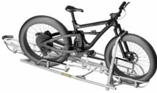
Figure 29: Sample Fat Tire Bike Tray for transit 4
