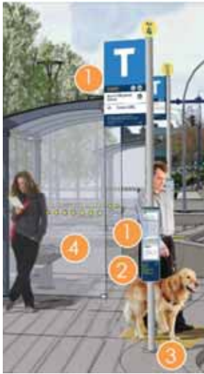
Figure 34: Elements of accessible bus stop, TransLink
