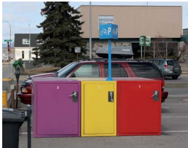
Class I bike parking refers to secure, weather-protected spaces intended for long-term use, typically either for residents of multi-family residences or employees. The bike parking in the Steele Street lot adjacent City Hall is an example of Class I bike parking.
