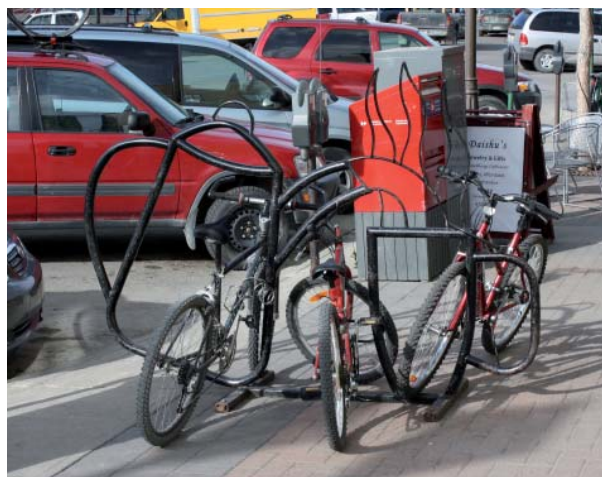
Class II bike parking refers to free-standing racks available to all cyclists with their own locking system, and are intended for short-term use. The rack at Main Street and 1st Avenue (right) is an example of Class II bike parking.
