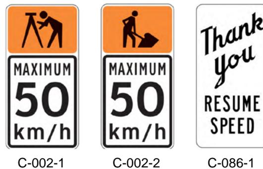
Figure 2.7: Typical Temporary Speed Zone Start and End Signage
