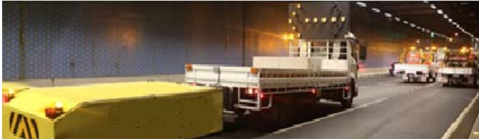
**Figure 4.32: Trailer-Style Crash Attenuator**
