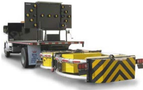
**Figure 4.33: Vehicle-Mounted Crash Attenuator**
