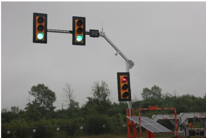
**Figure 4.22 C: Portable Traffic Signal with Countdown Timer – Green Display**
