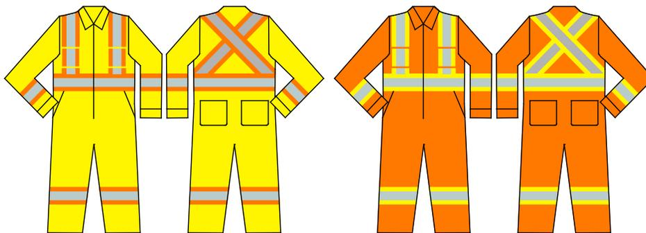
**Figure 5.3: Coveralls with Contrasting Retroreflective Bands**
