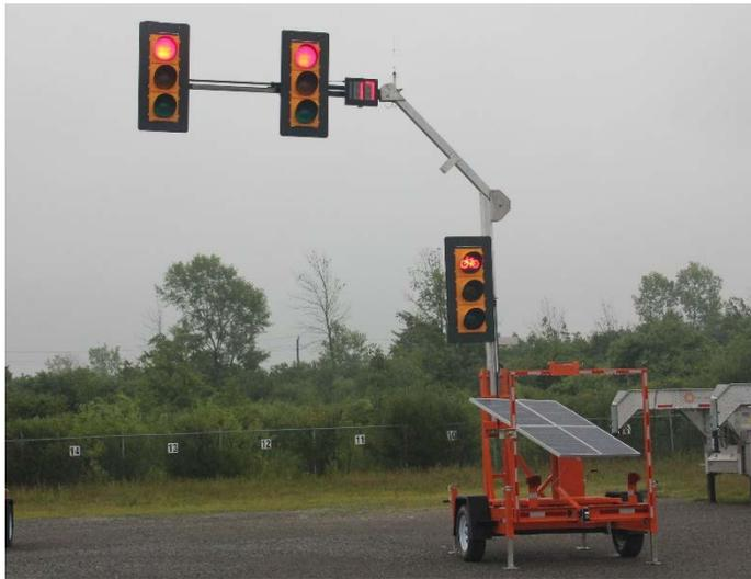
**Figure 4.22 B: Portable Traffic Signal with Countdown Timer – Red Display**
