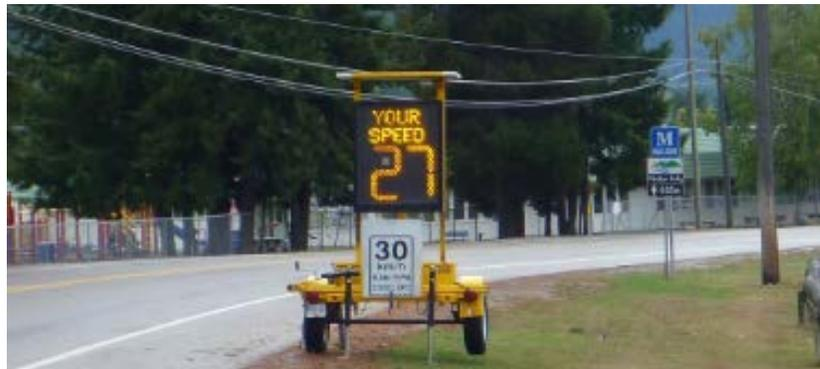
**Figure 4.28: Speed Reader Board**
